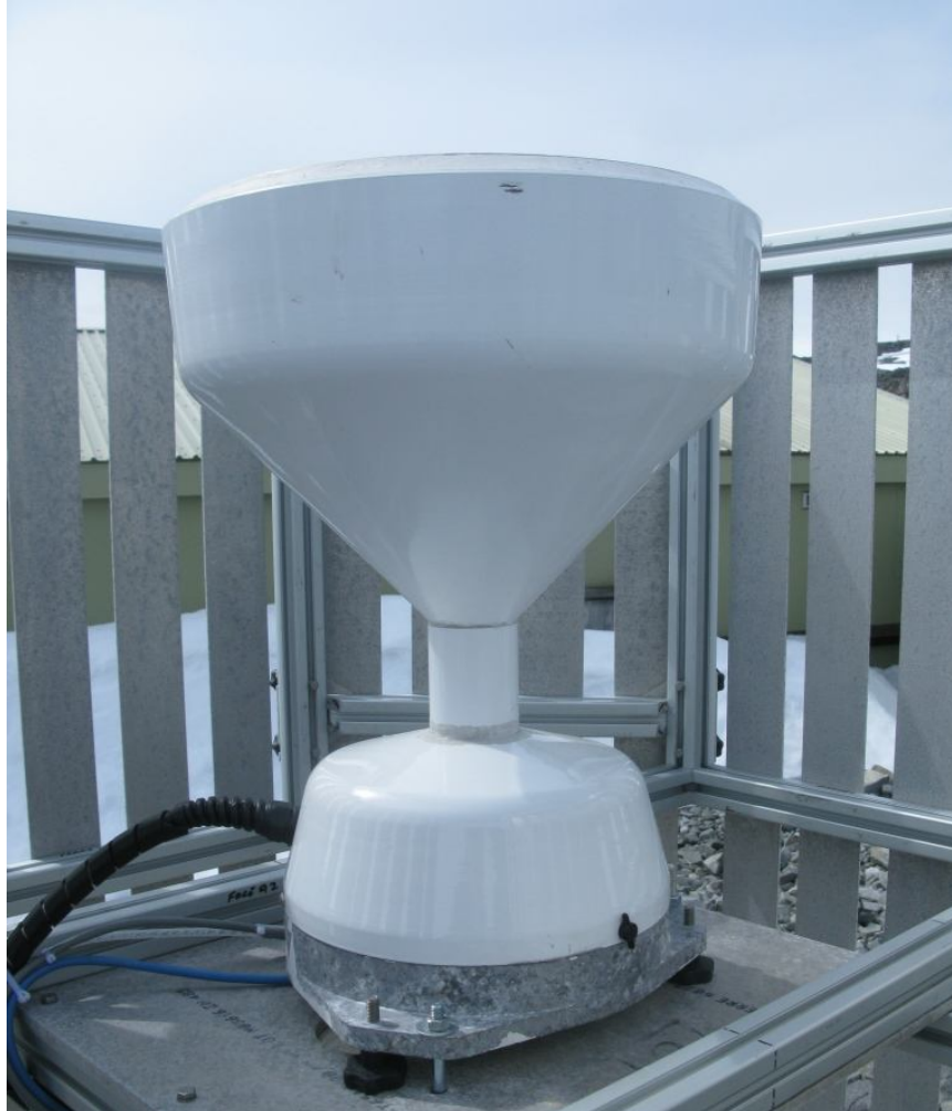
UPG1000 universal precipitation gauge with custom wind shield (Rothera, Antarctica courtesy BAS)
