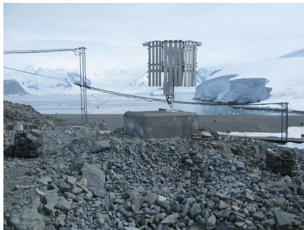
UPG1000 universal precipitation gauge with custom wind shield (Rothera, Antarctica courtesy BAS)
